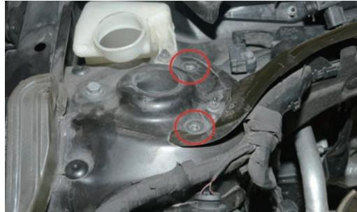
2. Place ② Washers onto the holes of strut mounts, then position ① Strut brace over the mounts and tighten the bolts back.
